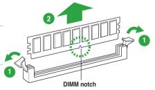
2. Remove the DIMM from the socket.
